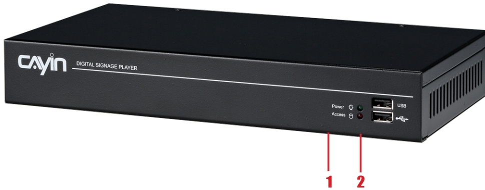
1. Power & HDD LED 2. Front USB connectors
