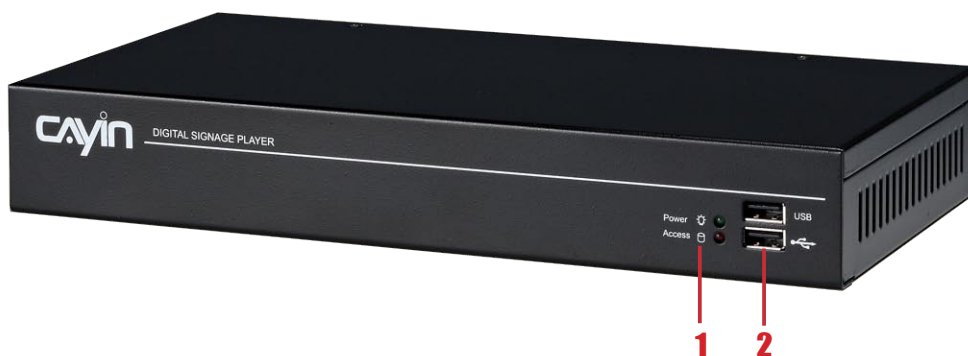
1. Power & HDD LED 2. Front USB connectors
