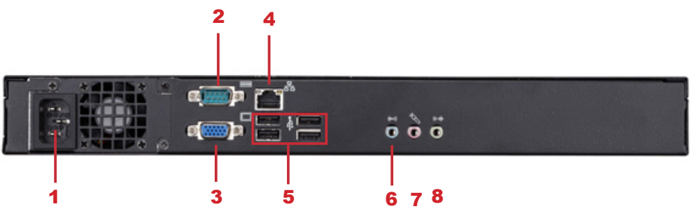
1. 电源接孔 2. RS-232 3. VGA 4. 以太网接孔 5. 4×USB 6. Line-In (预留) 7. Mic-In (预留) 8. Audio-Out
