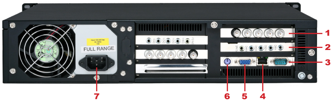
1. Video-In×4 (optional) 2. Line In×4 (optional) 3. COM 4. Ethernet 5. VGA 6. PS/2 7. Power Connector
