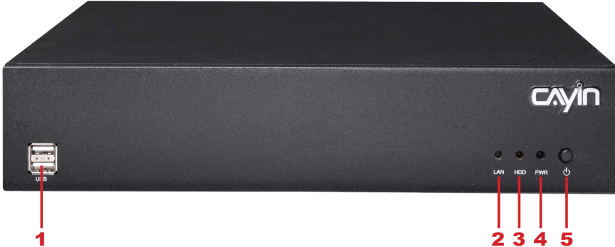
1. USB×2 2. Network Indicator 3. HDD Indicator 4. Power Indicator 5. Power
